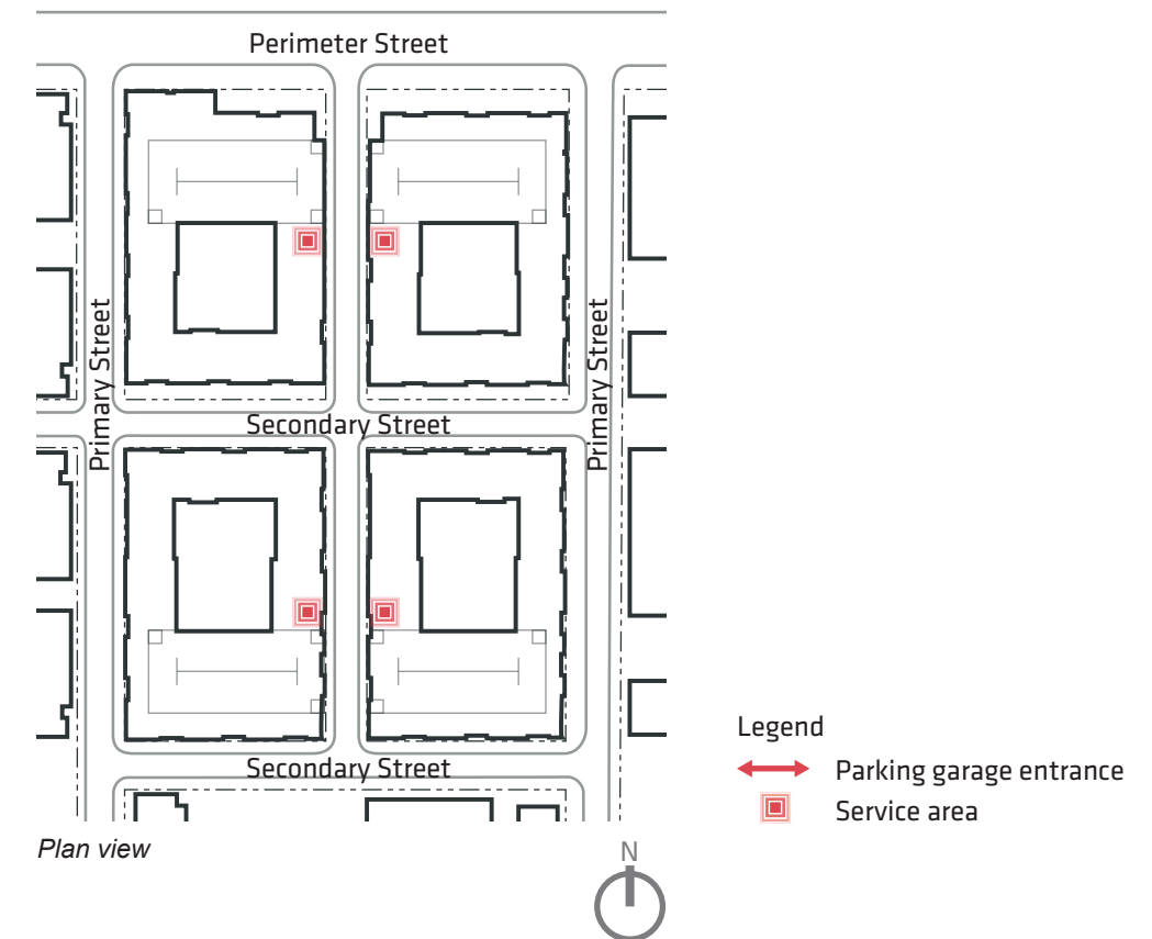
Building Service Access
